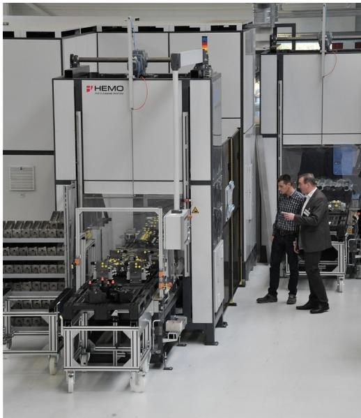
“ The hydraulic blocks enter the machine on plastic Euro pallets in any arrangement. To maximize output, two pallets can be stacked if needed. In this configuration, up to three tons of parts per hour can be cleaned to the highest quality, highlighting the superior performance of our system technology, ” explains HEMO CEO Andreas Fritz.
