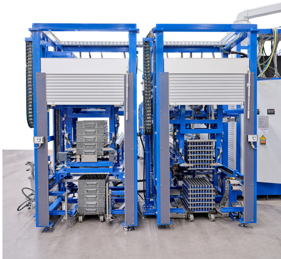
On the right side of the image is the loading station, and to the left of it is the parts removal area. Carts are used at both stations.
