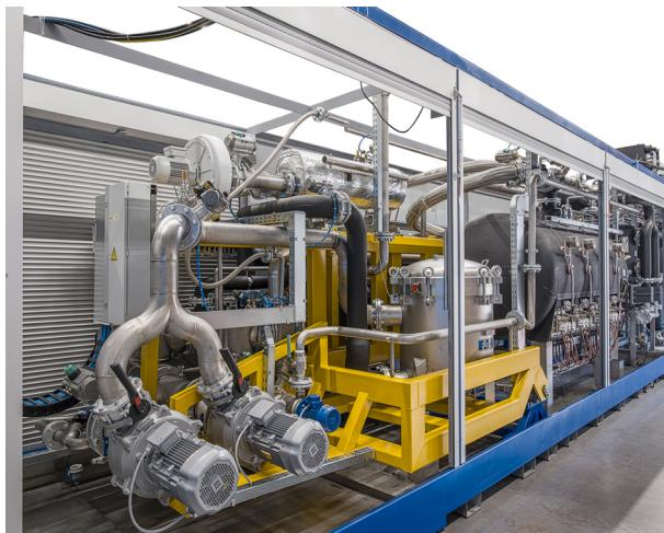
Two additional technical highlights significantly contribute to the exemplary cleaning quality of the system. In addition to ultrasonic assistance with 32 × 1.5 kW power, the cleaning chamber can be tilted by 4 - 10 degrees. This tilting of the basket significantly improves internal tube cleaning and, in combination with high-performance pumps, enables ultra-fast filling and emptying cycles — a crucial factor for completing the cleaning process within the short cycle time.
