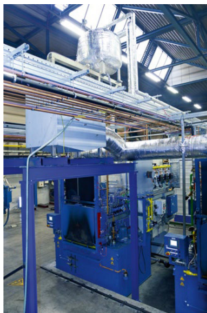
The waste heat from the hardening furnaces is used for heat recovery.
